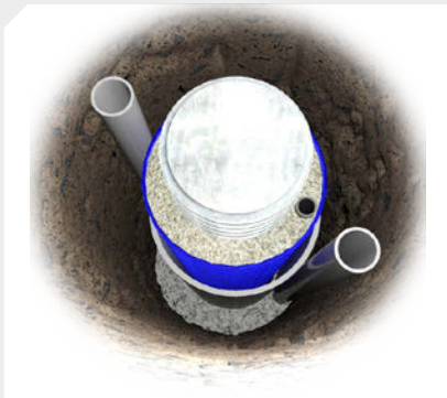
Cross-section of the free length of the anchor with an injection pipe
