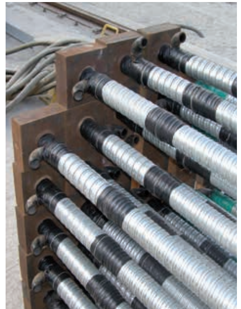
Prefabricated bar tendons
