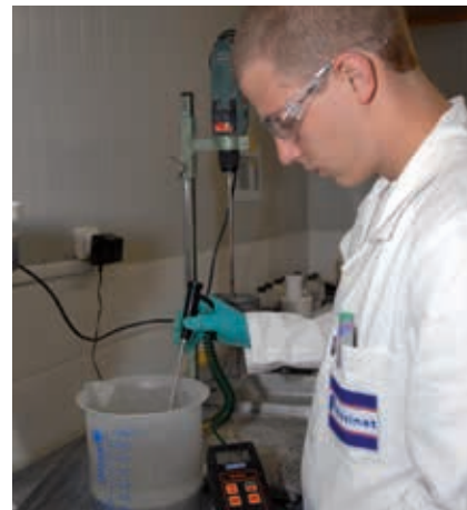
Formulation of cement grout in a Freyssinet laboratory
