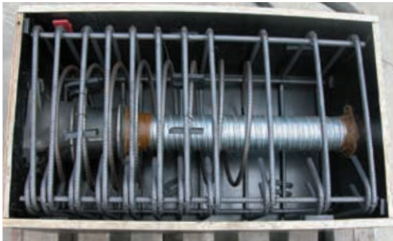
Reinforced concrete test prism for anti-burst test of 13C15 anchor
